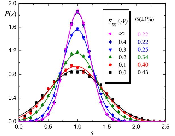
Fig. 5: (Color online) TWDs from simulated configurations (cf. fig. 4) with  $T = 723$  K and very small  $F = 0.01$  ML/s. The smooth curves are Gaussian fits, with the indicated standard deviations  $\sigma$ . With increasing  $E_{ES}$  the TWD evidently narrows ( $\sigma$  decreases).
