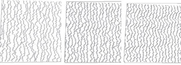
Fig. 4: Images of the simulated  $200 \times 1000$  vicinal surface after deposition of 20 ML for Ehrlich-Schwoebel barriers  $E_{ES}$ , from left to right: 0.1 eV, 0.3 eV, infinite. Other parameters are  $L = 10$ ,  $T = 723$  K,  $F = 0.01$  ML/s,  $E_d = 1.0$  eV, and  $E_a = 0.3$  eV.
