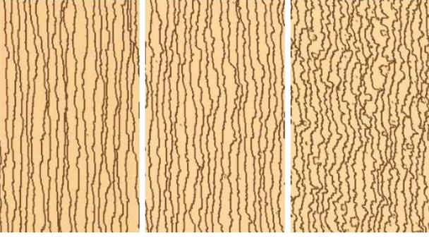
Fig. 1: (Color online) Images ( $200 \times 1000$  sites) of the vicinal surface after deposition of 150 ML for 3 growth rates (left to right): near equilibrium ( $F=0.1$  ML/s), moderate growth ( $F=1$  ML/s), and rapid growth ( $F=10$  ML/s) near the upper limit of step-flow growth.
