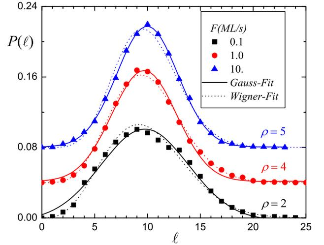
Fig. 2: (Color online) Simulated terrace-width distribution (TWD) for the 3 cases of fig. 1. The  $F = 1.0$  set is displaced upward by 0.4, the  $F = 10$  case by 0.8, for clarity. The solid curves show fits to a Gaussian, while the dotted curves are GWDs, eq. (1), for the indicated values of  $\varrho$ .
