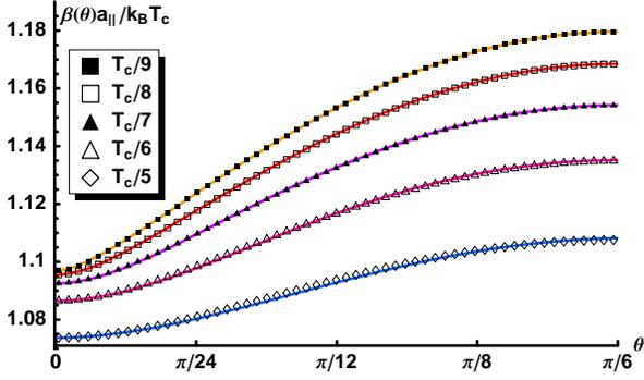
FIG. 3: (Color online) The orientation dependence of the explicit approximation for the  $\{111\}$  line tension (solid lines) is compared with the numerically evaluated exact result (symbols). Because of the six-fold symmetry, only the positive half of the first sextant is shown. (The negative half is mirror-symmetric.)
