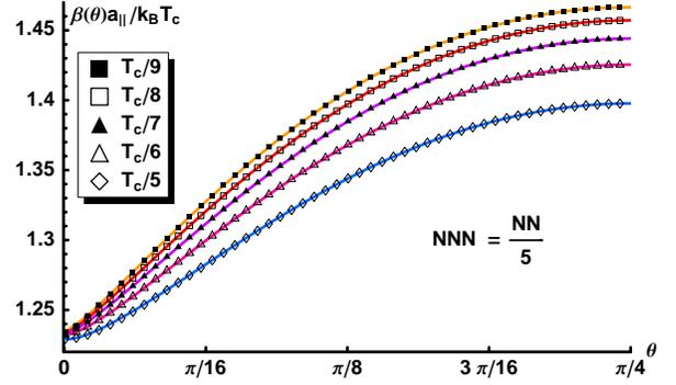
FIG. 5: (Color online) The orientation dependence of the explicit approximation for the  $\{001\}$  line tension (solid lines) is compared with the numerically evaluated exact result (symbols). Because of the four-fold symmetry, only the positive half of the first quadrant is shown (the negative half is mirror-symmetric).
