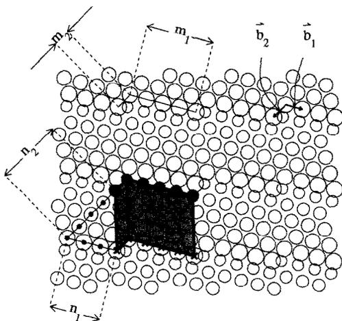
Fig. 2. Nomenclature for surfaces vicinal to (111), in this example (14109). Here  $m_1 = 4$ ,  $m_2 = 1$ ,  $n_1 = 3$ ,  $n_2 = 4$ . The bold lines outline the shaded (111) microfacet of a (14109) unit cell, in this example containing 19 unit cells, as discussed in the appendix.
