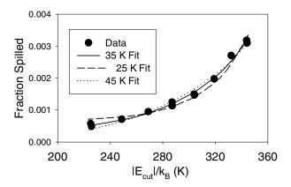
FIG. 3. Fraction of electrons spilled (f) versus  $E_{\rm cut}$  for a typical set of data (solid circles). Fits using the model based on Eq. (1) are shown for the temperatures that are indicated, where the 35 K curve is the best fit curve and the other two are shown for comparison. Note that the value of T is determined primarily from the curvature of f versus  $E_{\rm cut}$ .
