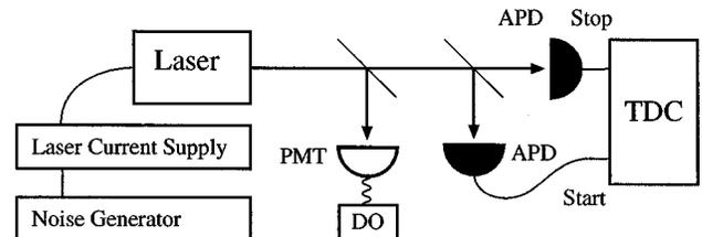
Fig. 2. Simplified diagram of the experimental setup.
