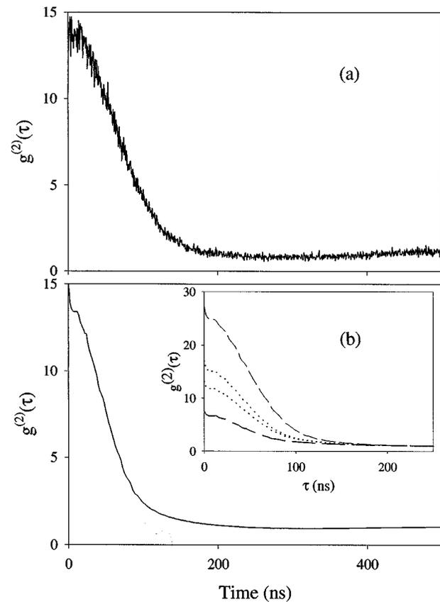
Fig. 9. Intensity correlation for noise modulation below threshold: (a) experiment and (b) simulation with  $i_0 = 37.3$  mA,  $i_{\text{thr}} = 59$  mA, and  $\beta = 0.91 \times 10^{-4}$ . The inset shows the sensitivity of the peak to changes in  $i_{\text{thr}}$  and  $\beta$ . The dashed curves are the curves with  $i_{\text{thr}} \pm 2\%$ . The dotted curves show the effect of varying  $\beta$  by  $\pm 10\%$ .
