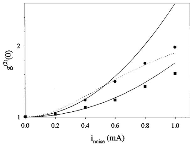
Fig. 7. Bunching as a function of applied noise current. The circles (squares) are the measured values of  $g_s^{(2)}(0)$  for the noise modulation passing through a 2.6-MHz (1.2-MHz) low-pass filter. The solid curves are predictions based upon the linear model outlined above with no adjustable parameters. The dotted curve is a calculation with the nonlinear model ( $\beta = 1.0 \times 10^{-4}$ ,  $i_{\text{thr}} = 59$  mA).
