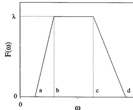
Fig. 1. Model spectral density of the noise source with five parameters  $a, b, c, d$ , and  $\lambda$  to specify the spectrum and its Fourier transform.
