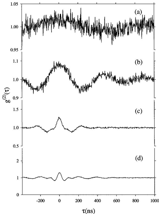
Fig. 4. Experimental plots of the correlation function for different bandwidths of the noise source and the laser operating below threshold,  $i = 56$  mA: (a) 1.2-MHz low-pass filter, (b) 2.6-MHz low-pass filter, (c) no filter, and (d) 6-MHz high-pass filter. Note the different vertical scales.
