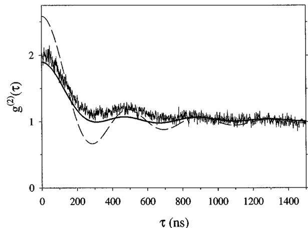
Fig. 6. Bunching for  $i_{\text{noise}} = 1$  mA filtered with the 2.6-MHz low pass. The continuous curve is a theoretical calculation based on the nonlinear model. The dashed curve is the prediction of the linear model with  $a = b = 0$ ,  $c = 2.25$  MHz,  $d = 2.75$  MHz, and  $i_{\text{noise}} = 1$  mA.
