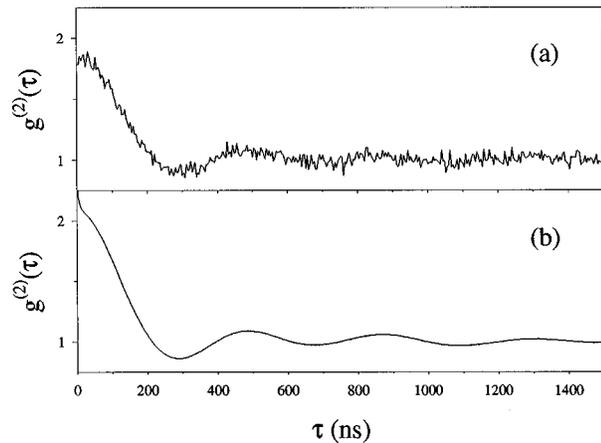
Fig. 8. Comparison of  $g_s^{(2)}(\tau)$  from (a) photon counting and (b) from a time series of intensities measured with a single PMT.
