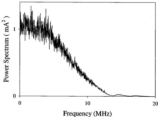
Fig. 3. Measured power spectrum of the 10-MHz-wide noise source at the current supply output.  $\Delta f = 20$  kHz.
