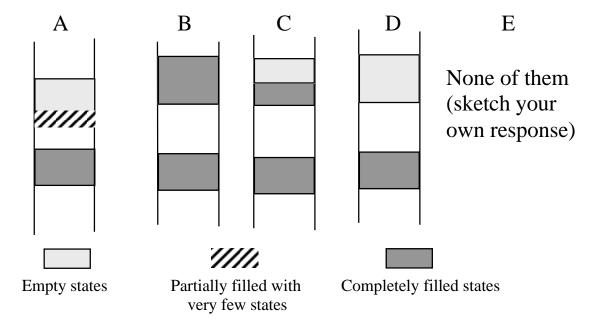
a. Consider the following band diagrams. For the each of the materials listed below the diagram, select the diagram that best represents the band structure of the material. For each material, **explain how you arrived at your answer.**
