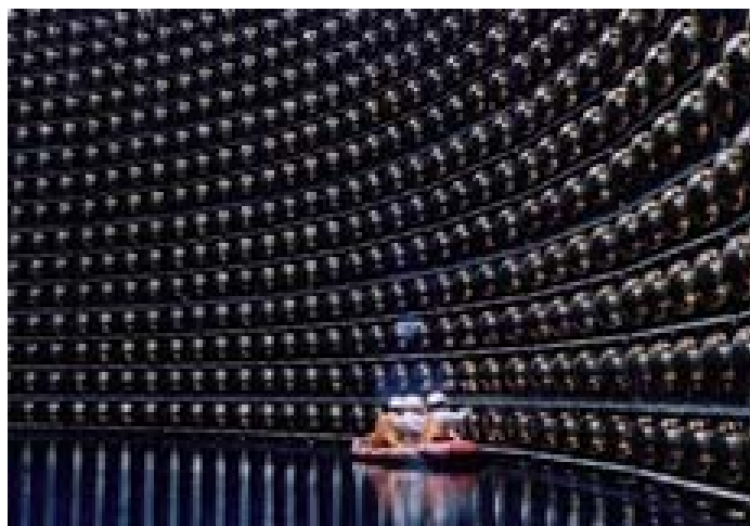
Fig. 2: The Super-Kamiokande detector is a tank holding 50,000 tons of water and surrounded by over 11,000 photomultiplier tubes (PMTs). When a neutrino interacts in the water, a cone of light is seen by the PMTs. In this picture workers are cleaning the PMTs as the tank slowly fills with water. The University of Maryland played a leading role in the experiment, which offered the first conclusive evidence for neutrino mass.
