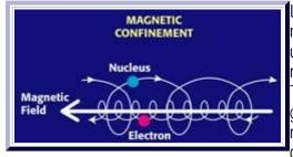
Luckily, we can use magnetic fields. A charged nucleus at a 100M-degree temperature, if unimpeded, will zip across a few meters in a microsecond. Put the same nucleus in a one Tesla magnetic field and the nucleus will simply gyrate around the field line with a radius of a few mm. We thus have containment – except for one detail: while the nucleus performs a tight circle
