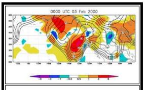
The chaos group at the University of Maryland is working to improve weather forecasts. Colors show the improvement in a forecast (in surface pressure) compared to conventional forecasting techniques when the information about the local complexity of the atmosphere (contours) is used.
