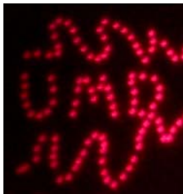
Fig. 3: Larger view of the custom pattern of laser focal points of the adaptive tweezer system applied to a dyed fluid sample.
