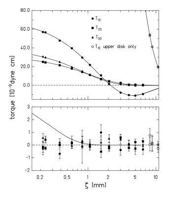
Figure 2: Upper panel: torques measured in the first experiment of Hoyle et al. as a function of pendulum/attractor separation. Open circles are data taken with the lower attractor disk removed and show the effect of uncancelled gravity. Smooth curves show the Newtonian fit. Lower panel: residuals for the Newtonian fit. The solid curve shows the expected residual for a Yukawa force with  $\alpha = 3$ and  $\lambda = 250 \ \mu$ m.
