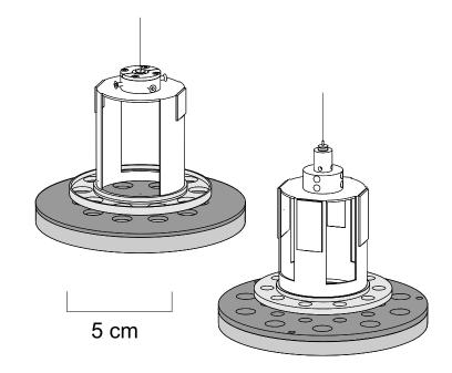
Figure 1: Schematic diagram of the 10-hole pendulums and rotating attractors used in the two experiments of Hoyle et al.(69, 145, 146). The active components are shaded.
