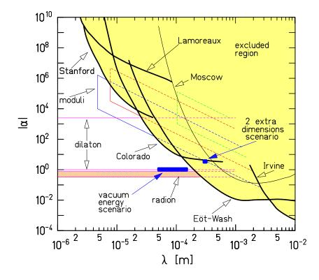
Figure 6: 95% confidence level constraints on ISL-violating Yukawa interactions with  $1\mu m < \lambda < 1$  cm. The heavy curves give experimental upper limits (the Lamoreaux constraint was computed in Ref. (148)). Theoretical expectations for extra dimensions(54), moduli(98), dilaton(99) and radion(80) are shown as well.
