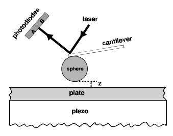
Figure 7: Schematic diagram of the Casimir-force apparatus used in Ref. (162)
