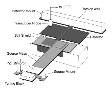
Figure 3: Schematic diagram of the instrument used by Long et al.(138).
