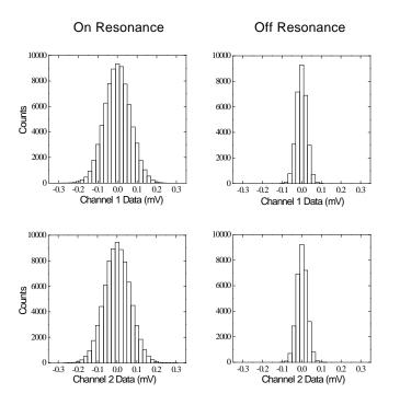
Figure 4: Data from the experiment of Long et al.(138) showing the two quadrature signals from the torsion oscillator.
