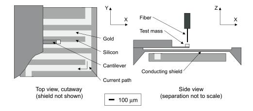
Figure 5: Schematic diagram of the instrument used by Chiaverini et al.(149)
