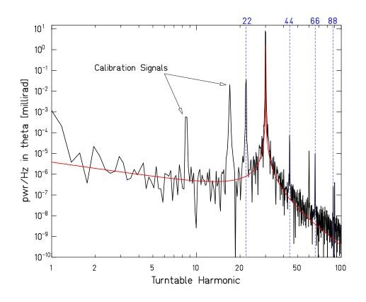
Figure 10: Spectral density of the torque signal in the 22-fold symmetric experiment of the Eöt-Wash group. The peaks at 8.5 and 17  $\omega$  are gravitational calibrations; the fundamental and first three overtones of the short-range signal are at 22, 44, 66, and 88  $\omega$ . The smooth curve shows the thermal noise computed using Eq. 33.
