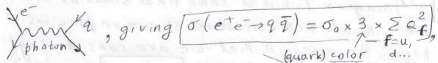
where we simply re-cycle (with appropriate modifications as shown) the  $e^+e^- \rightarrow \mu^+\mu^-$  calculation, i.e.,
