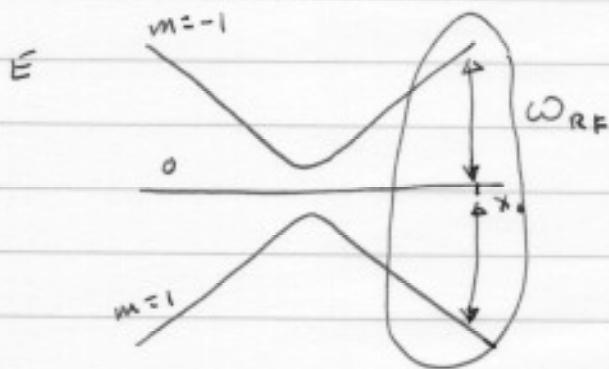
apply  $\omega_{RF}$  so  $\hbar\omega_{RF} = \mu B(x_0)$
