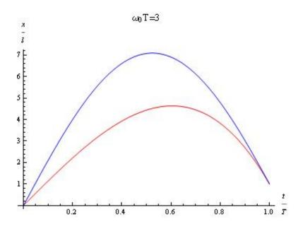
where the red plot is our function x(t), and the blue one is the exact solution of the system (which is obtained from *Problem 3*). From the plot we can see that the function x(t) cannot give us a good approximation if  $\omega_0 T \to 3$ , where the reason is, as stated in *part c*) before, the second differentiation of action S(c) tends to zero when  $\omega_0 T \to \sqrt{21/2}$ , which makes our approximation 'not good enough' to represent the exact solution.
