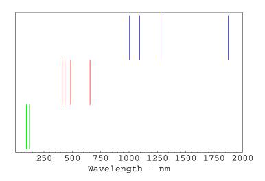
2. Another interesting property of the hydrogen wavelengths is known as the *Ritz combination principle*. If we convert the hydrogen emission wavelengths to frequencies, we find the curious property that certain pairs of frequencies added together give other frequencies that appear in the spectrum! Show that the longest wavelength of the Balmer series and the longest two wavelengths of the Lyman series satisfy the Ritz combination principle.
