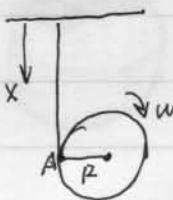
Suppose Yo-Yo roll about its origin a cycle, then the contacting point of the Yo-Yo with the vertical line is still the point A on Yo-Yo, so we get
