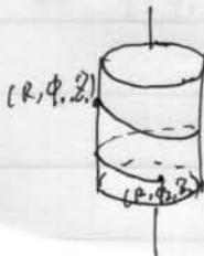
In cylinder coordinates, when  $R$  is const, the infinitesimal change in position corresponds to  $ds = \sqrt{R^2 d\phi^2 + (dz)^2} = d\phi \sqrt{1 + R^2 \dot{\phi}^2} = f(\phi', z) d\phi$
