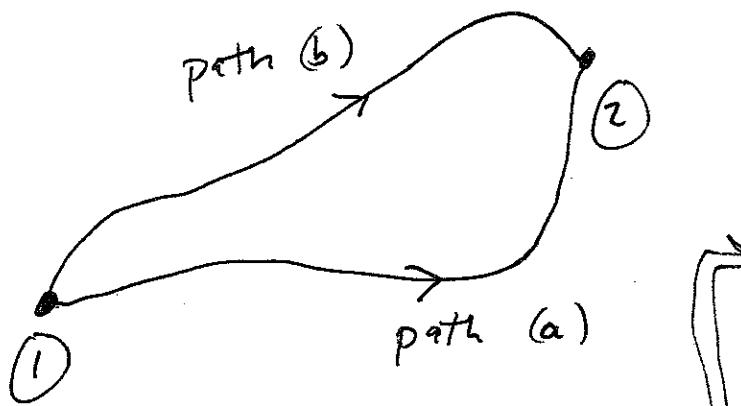
$$\text{Then } W_{12} = \int_{\text{path a}} \vec{F} \cdot d\vec{r} = \int_{\text{path b}} \vec{F} \cdot d\vec{r}$$
