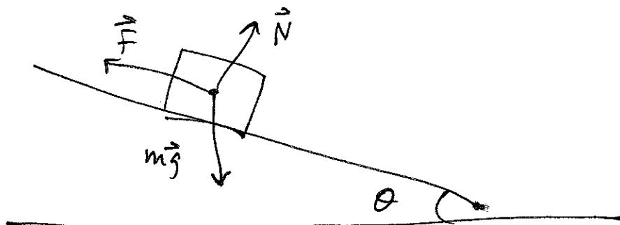
For a uniform gravitational field,  $\vec{F}_{\text{gravity}} = -mg\hat{z}$ ,
