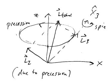
If I is large enough, then the x components of Le & Lz cancel, and then I is almost entirely vertical. In this case there is no torque, so we have free precession of êz about I
