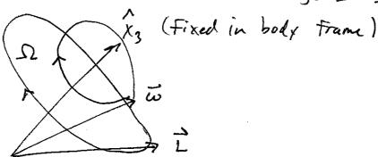
In space the space frame, a fixed, inertial coordinate system, I is constant (because there is no torque), and  $\hat{x}_3$  and  $\hat{w}$  precess about it.
