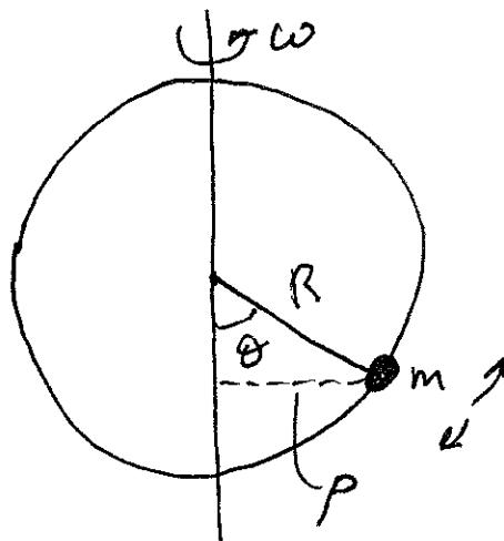
The bead is free to move up and down the hoop with angle  $\theta$ . It also rotates in the plane around the axis of the hoop.
