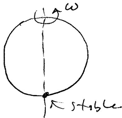
But if the speed increases, with  $\omega^2 \geq g/R$ , then the bottom position becomes unstable, but two stable equilibria appear on either side of the hoop:
