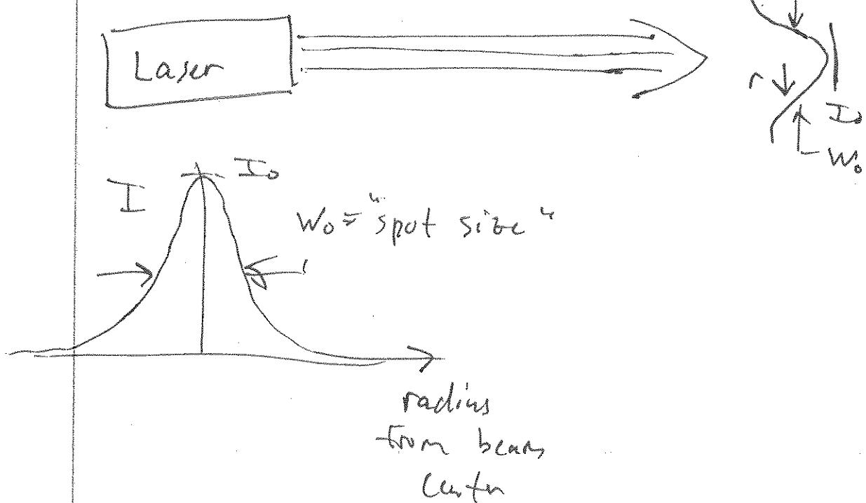
It is possible to measure the focal length of a lens by measuring the expansion or contraction of the beam width:
