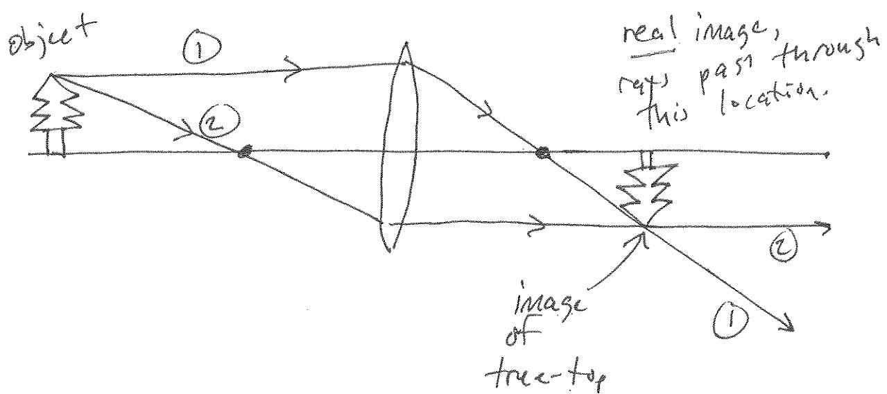
6) To confirm the image location, draw the 3<sup>rd</sup> principle ray, which passes through the center of the lens ~~and~~ and is un-diverted. (because the two sides of the lens glass are parallel in the center, so the ray jogs over very slightly but does not bend.)
