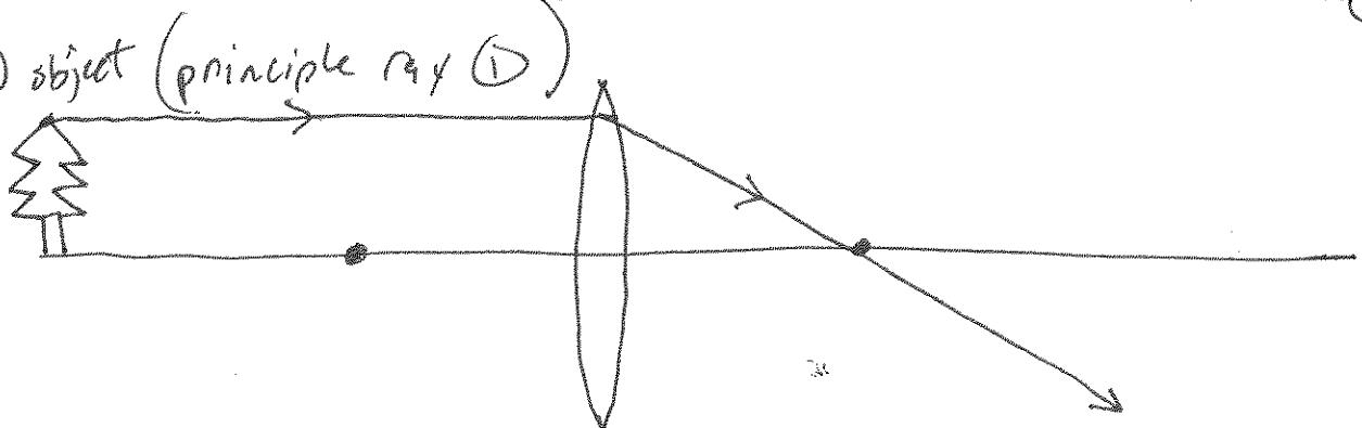
Draw principle ray ①, which departs from the top of the tree traveling parallel to the optical axis. This ray will be diverted by the lens to pass through the focal point on the other side.
