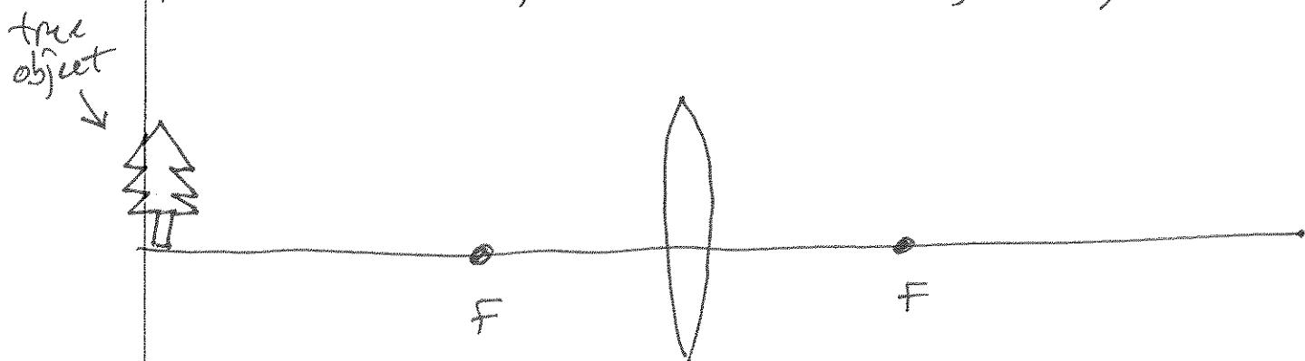
The base of the tree sits on the optical axis, and the image of the base will also be on the optical axis. Our goal is to determine where the top of the tree will be imaged.
