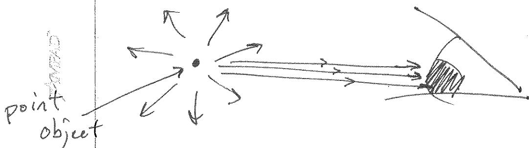
An optical system collects some of the light and re-directs the rays to a 2<sup>nd</sup> location, simulating what the object would look like if it were located there:
