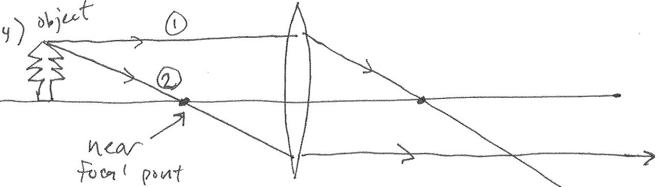
Draw Principle Ray ②, which departs from the top of the tree and passes through the near focal point. This ray is diverted by the lens to travel parallel to the optical axis.
