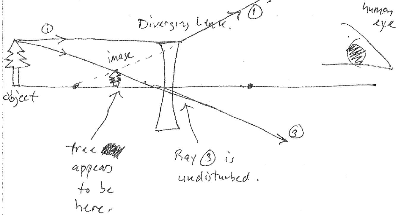
$$\text{Thin Lens Equation: } \frac{1}{s} + \frac{1}{s'} = \frac{1}{f}$$
