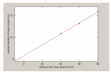
If  $I = I_0 e^{-\frac{2r^2}{w^2}}$ , and Gaussian form is  $I = I_0 e^{-\frac{r^2}{2\sigma^2}}$ , then  $w = 2\sigma$ . The divergence angle  $\theta$  is then given by 2\*atan(2\*slope). Reasonable values are in the range 2x10<sup>-3</sup> rad (~0.1 degree).
