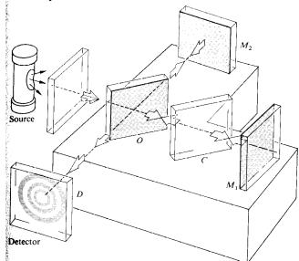
Start with the laser at a fixed height, the beam aligner at a fixed height, the front of the MI at a fixed height and level. (If the heights are messed up, have Tommy reset them.) Then adjust the mirror on the beam aligner to retroreflect. Use the two knobs on the back of the mirror, and adjust the beam height using the knob on the side of the unit. You must both retroreflect the beam and center the beam on the moveable mirror in the MI.
