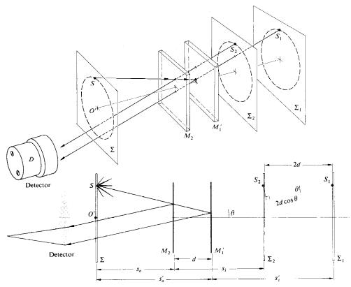
Destructive interference occurs when the path length difference is an integer number of wavelengths:
