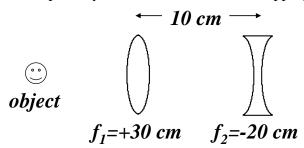
For the first lens  $1/s_{i1} = 1/f \cdot 1/s_{o1} = 1/30 \cdot 1/30 = 0$ ,  $s_{i1} = infinity$ .  $s_{i1}$  becomes  $s_{o2}$  at – infinity. Thus,  $1/s_{i2} = -1/20 + 1/infinity = -1/20$ ,  $s_{i2} = -20$  cm. The image is virtual and 10 cm in front of the first lens. The magnification of for the system is  $M = (s_{i1}/s_{o1})(s_{i2}/s_{o2}) = (-infinity/30)(20/-infinity) = 2/3$ .
