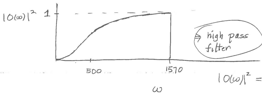
$$\begin{aligned} RC &= (1000)(2 \times 10^{-6}) \\ &= 2 \times 10^{-3} \\ \frac{1}{RC} &= 500 \end{aligned}$$
