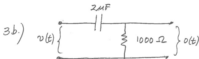
$$\left. \begin{array}{l} V(\omega) - \frac{Q(\omega)}{C} - RI(\omega) = 0 \\ Q(\omega) = RI(\omega) \\ -i\omega Q(\omega) = I(\omega) \end{array} \right\} \Rightarrow O(\omega) = \frac{R}{R + \frac{1}{i\omega C}} V(\omega) = \frac{\omega V(\omega)}{\omega + \frac{i}{RC}}$$
