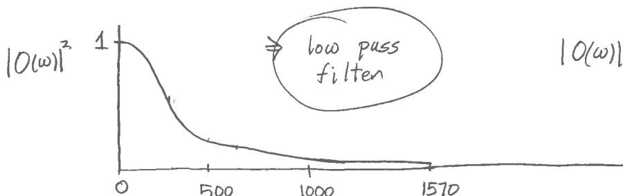
$$|O(\omega)|^2 = \frac{(R/L)^2 |V(\omega)|^2}{\omega^2 + (R/L)^2} = \frac{(250)^2}{\omega^2 + (250)^2}$$
