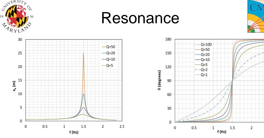
• x<sub>0</sub> is max at a special frequency: <u>resonance</u>
