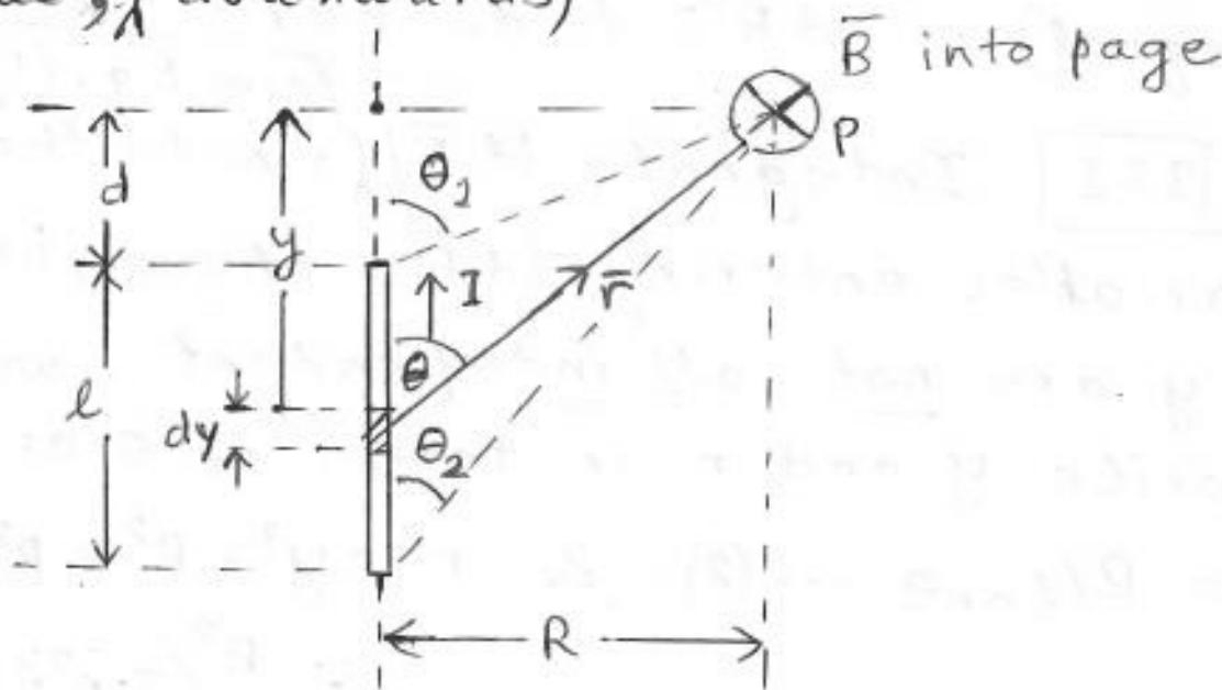
Step "0": draw neat figure (as above), showing direction of  $d\vec{B}$  (magnetic field) due to element  $dy$ , i.e., into page (using RH rule, i.e.,  $d\vec{I}$  is upward -
