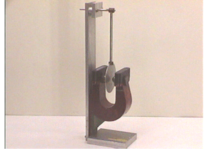
K2-44: EDDY CURRENT PENDULUM
