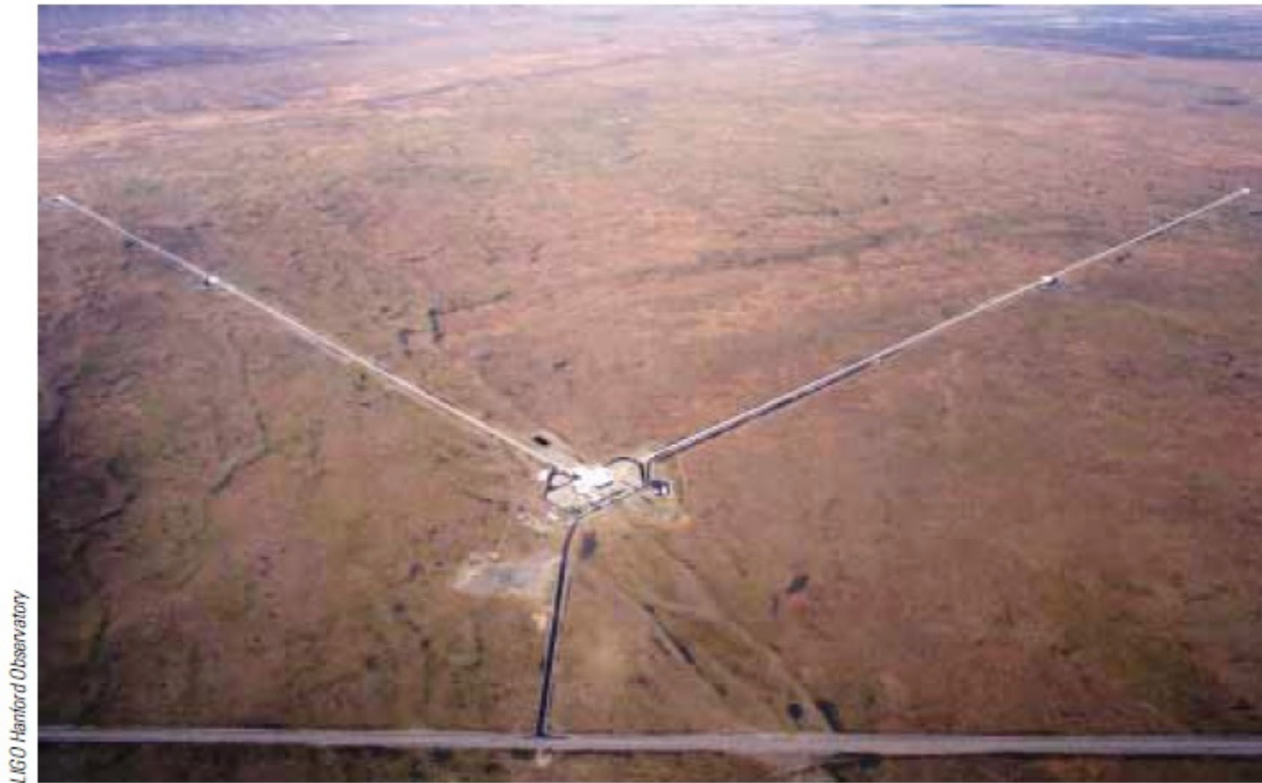
Figure 37.23 The Laser Interferometer Gravitational-Wave Observatory (LIGO) near Richland, Washington. Note the two perpendicular arms of the Michelson interferometer.
