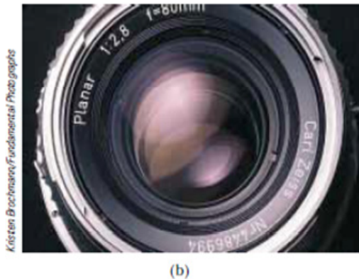
Figure 37.20 (Example 37.4) (a) Reflective losses from a silicon solar cell are minimized by coating the surface of the cell with a thin film of silicon monoxide. (b) The reflected light from a coated camera lens often has a reddish-violet appearance.
