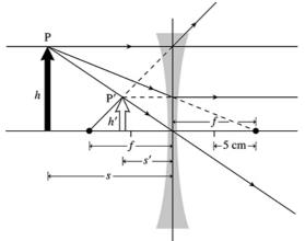
The figure shows the ray-tracing diagram using the steps of Tactics Box 23.3. The three rays after refraction do not converge at a point, but they appear to come from P'. P' is 6 cm from the diverging lens, so s' = -6 cm. The image is upright.
