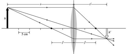
The figure shows the ray-tracing diagram using the steps of Tactics Box 23.2. You can see from the diagram that the image is in the plane where the three special rays converge. The image is located at s' = 15 cm to the right of the converging lens, and is inverted.
