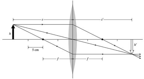
The figure shows the ray-tracing diagram using the steps of Tactics Box 23.2. You can see from the diagram that the image is in the plane where the three special rays converge. The image is inverted and is located at s' = 20.0 cm to the right of the converging lens.
