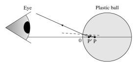
**Solve:** The bubble is at P, a distance of 2.0 cm from the surface. So, s = 2.0 cm. A ray from P after refracting from the plastic-air boundary bends away from the normal axis and enters the eye. This ray appears to come from P', so the image of P is at P' and it is a virtual image. Because P faces the concave side of the refracting surface, R = -4.0 cm. Furthermore,  $n_1 = 1.59$  and  $n_2 = 1.0$ . Using Equation 23.21,
