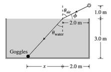
The laser beam enters the water 2.0 m from the edge, undergoes refraction, and illuminates the goggles. The ray of light from the goggles then retraces its path and enters your eyes. **Solve:** From the geometry of the diagram,
