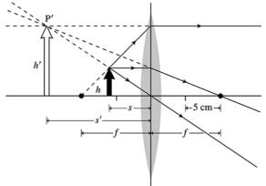
The figure shows the ray-tracing diagram using the steps of Tactics Box 23.2. You can see that the rays after refraction do not converge at a point on the refraction side of the lens. On the other hand, the three special rays, when extrapolated backward toward the incidence side of the lens, meet at P', which is 15 cm from the lens. That is, s' = -15 cm. The image is upright.
