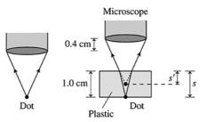
**Solve:** When the plastic is in place, the microscope focuses on the virtual image of the dot. From the figure, we note that s = 1.0 cm and s' = 1.0 cm - 0.4 cm = 0.6 cm. The rays are paraxial, and the object and image distances are measured relative to the plastic-air boundary. Using Equation 23.13,
