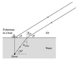
A ray that arrives at the diver 50° above horizontal refracted into the water at  $\theta_{water} = 40^{\circ}$ . Solve: Using Snell's law at the water-air boundary
