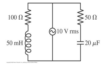
When the frequency is very small,  $X_c = 1/\omega C$  becomes very large and  $X_L = \omega L$  becomes very small. So, the branch in the circuit with the capacitor has a very large impedance and most of the current flows through the branch with the inductor. When the frequency is very large, the reverse is true and most of the current flows through the branch with the capacitor.
