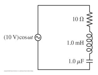
**Solve:** (a) The resonance frequency of the circuit occurs when the reactance of the capacitor is the same as that of the inductor hence the voltage is in phase with the current. The resonant frequency is given by,
