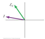
Current leads the voltage which implies that capacitive reactance is more than the the inductive reactance. Now we have the capacitive reactance behaving inversely with frequency and inductive reactance behaving directly with frequency, hence frequency has to be less than the resonant frequency to increase the  $X_c$  and decrease  $X_L$
