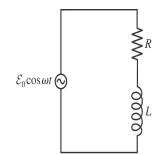
Visualize: Series elements have the same current, so we start with a common current phasor I for the inductor and resistor,
