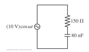
**Model:** The current and voltage of a resistor are in phase, but the capacitor current leads the capacitor voltage by 90°. **Solve:** THe reactance of the resistor is R wereas for the capacitor it is given by,
