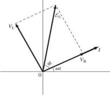
**Solve:** Because we have a series RL circuit, the current through the resistor and the inductor is the same. The voltage phasor  $V_{\rm R}$  is along the same direction as the current phasor *I*. The voltage phasor  $V_{\rm L}$  is ahead of the current phasor by 90°.
