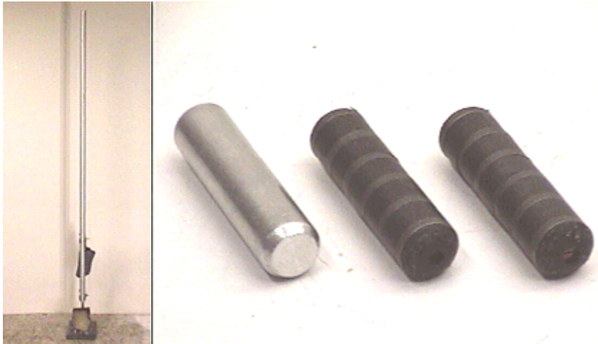
K2-42: LENZ'S LAW - MAGNET IN ALUMINUM TUBE
