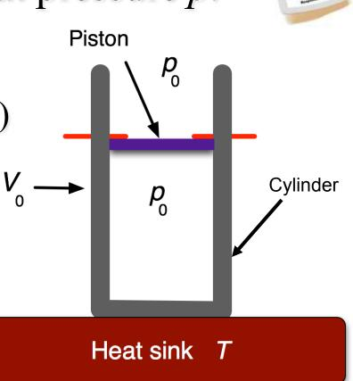
If we pull the pins holding the piston in place, the gases would expand until the pressures are equal. What would the new volume be?
