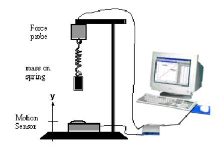
A mass is hanging from a spring. The position of the mass is measured by a sonic ranger sitting 25 cm under the mass's equilibrium position. At some time, the mass is started oscillating.
