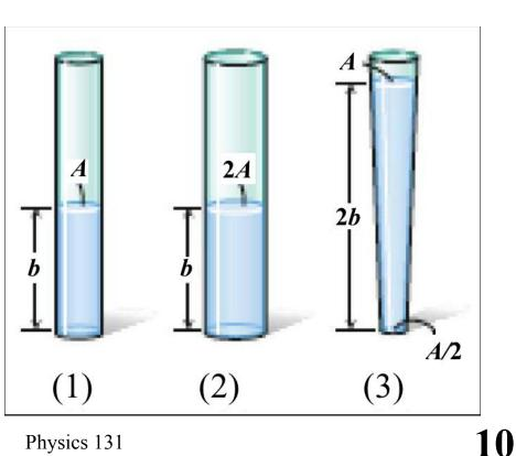
Consider the containers at right. Which of the following correctly compares the *force* (F) exerted by the water on the bottoms of the containers?
