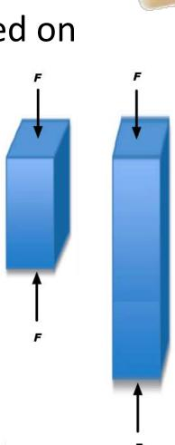
Consider two blocks made of the same material with the same length but one twice cross sectional area as the other. If the same compressional forces are exerted on both blocks
