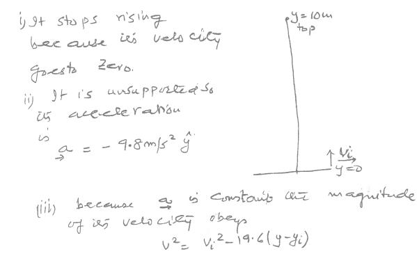
Since y'=0, and at ytop, v=0.  $0 = v_i^2 - 19.6 \text{ m/s}$   $v_i = \sqrt{146} \text{ m/s}$   $v_i' = + 14 \text{m/s} \hat{y}$
