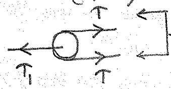
Since it is the same rope (assumed massless) that goes around the pulley, the tension in both segments of the rope is assumed to be the same.
