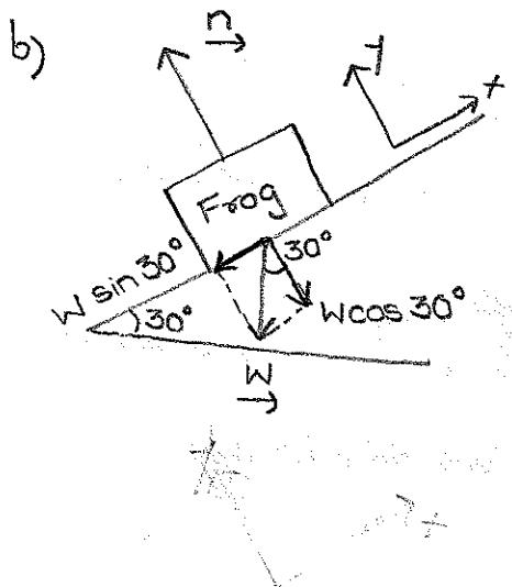
As shown in figure, I choose my x and y-axis along and perpendicular to the incline.
