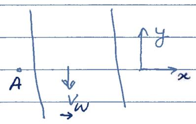
speed with respect to the water is  $0.5 \text{ m/s}$  (no matter what the direction) what direction would you go so as to land directly opposite to the point A? What would your velocity be with respect to the shore.
