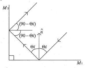
And from the figure above you can see that after the two reflections the light follows a path which is anti-parallel to the incident ray.
