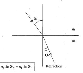
Product of refractive index and sine of the angles with respect to normal is a constant.
