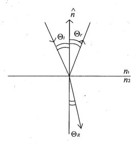
So now light is arriving at angle  $\Theta_i$ . Fermat's principle controls the angles  $\Theta_r$  (reflected ray) and  $\Theta_R$  (refracted ray).
