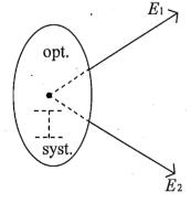
$E_1$ ,  $E_2$  are diverging so they will not intersect. You will have to extrapolate the  $E_1$ ,  $E_2$  lines to locate the image  $\mathbb Z$  as the point from which  $E_1$ ,  $E_2$  "appear" to be coming. No light actually goes through  $\mathbb Z$  so it is called a VIRTUAL IMAGE
