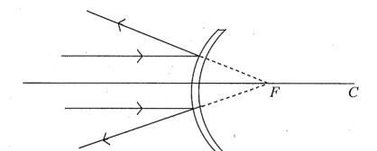
A parallel beam of light incident on a convex mirror, on reflection appears to start from F and becomes divergent.
