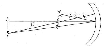
V' p = f, object at  $F, q \to \infty$ ,  $m \to \infty$ Point source at F on reflection
