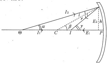
Same construct.  $I_1, I_2$  start from 0, after reflection we get  $E_1, E_2$ , intersection locate I.
