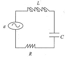
To work out behavior of L-C-R circuit we have to keep track of the relative phases in R, C, and L.
