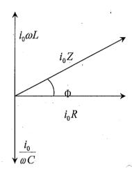
$$\varepsilon_0 = v_0 = i_0 \left[ R^2 + \left( \omega L - \frac{1}{\omega C} \right)^2 \right]^{\frac{1}{2}}$$
