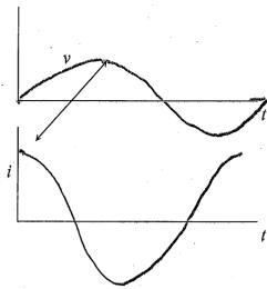
$\frac{1}{\omega C}$  has dimensions of R and we define capacitive reactance
