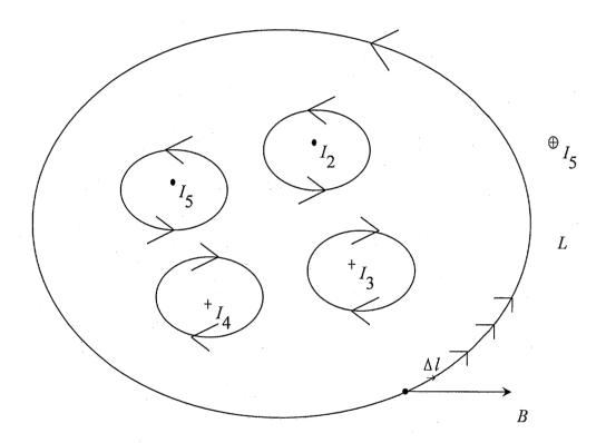
Repeat this calculation at every step as shown.  $B_1 \bullet \Delta l_1 + B_2 \bullet \Delta l_2 + B_3 \bullet \Delta l_3 + \dots$ Write out the sum
