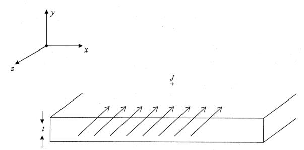
At y=0 there is a Current sheet of thickness t carrying current density  $J=-J\hat{z}$ . Looking it endon we see sources of B as
