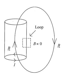
4.) <u>Hollow Cylindrical Conductor</u>- Radius R, carries uniform current. We want  $\stackrel{B}{\rightarrow}$  at a distance r from its axis. Since there is a cylindrical symmetry we should use circles centered on the axis for our closed loop. For r < R, use loop 1.
