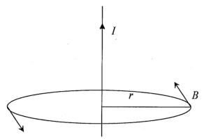
Single wire with current I, there is cylindrical symmetry so B can be a function of r only & must encircle I. [B and  $\Delta I$  are parallel to one another.]
