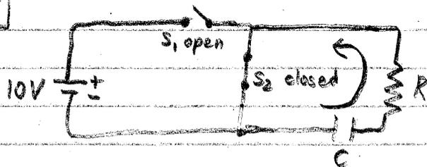
The capacitor will now discharge via  $S_2$ , without being charged via the battery and  $S_1$ .
