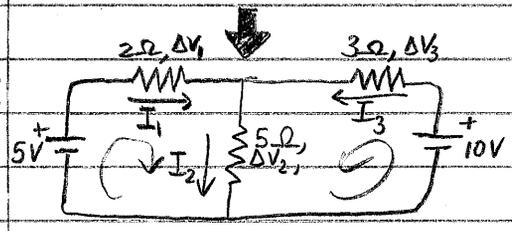
First, we need to have labels for all the things we'll need to calculate: currents  $I_1$ ,  $I_2$ , and  $I_3$ , and potential drops  $\Delta V_1$ ,  $\Delta V_2$ , and  $\Delta V_3$ .
