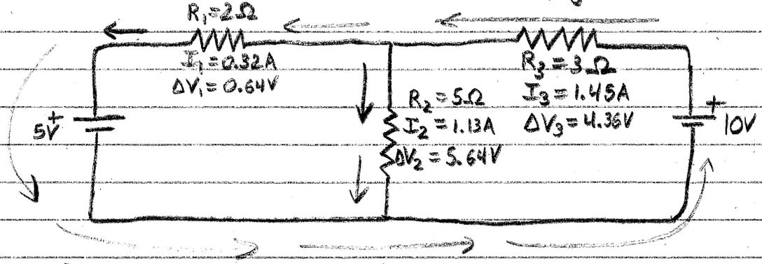
Flow of current marked with arrows. You can check these numbers by plugging them back into equations (i) through (vi)
