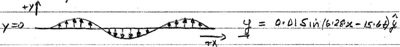
This is a transverse wave - displacement is perpendicular to the line of travel.
