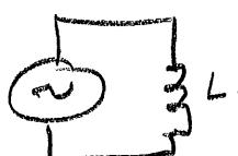
$$E - L \frac{\Delta I}{\Delta t} = 0 \text{ so } V \text{ and } \frac{\Delta I}{\Delta t} \text{ are in phase}$$
