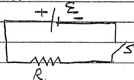
When you close the switch S the battery drives a current through R
