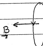
a single ring with current as shown will produce a field along  $\hat{x}$ - $\hat{x}$  on its axis.
