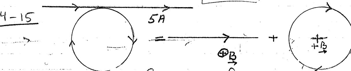
Straight wire with loop = Superposition of straight wire and one loop,
