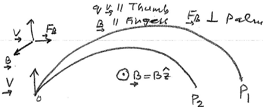
As shown, for charges to turn right at the origin, force  $\vec{F}_B$  must be along  $+x$ , since  $\vec{F}_B = q[\vec{v} \times \vec{B}]$  we need  $\vec{v} \parallel$  along  $+y$ , hence  $q$  must be positive.
