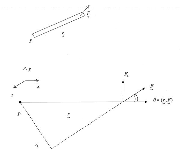
Notice that in turning the bar about an axis through P, only component of  $F \perp r$  matters or alternatively, the moment arm  $r_{\perp}$  controls  $\tau$ .
